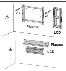
The Wall Mounting Unit should be mounted to a wall that can adequately hold the total weight of the plasma/LCD display and the Wall Mounting Unit over a long period of time and which can adequately withstand earthquakes, conceivable vibrations, and other external forces. Improper installation may cause the Plasma/LCD display to fall down, resulting in physical injury.
